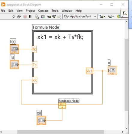
Her is the LabVIEW implementation of our Integrator. Basically, we can use this for all kind of differential systems, either we have one or many differential equations. Here is a Formula Node used, but you could have used pure LabVIEW code as well
